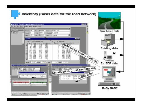
Inventory data or the basic geometric data is entered to RoSy BASE in e.g. below files (windows). The registration may be done manually and/or digitally from other recording systems or already existing databases. The data entered to RoSy can of course also be applied by other systems.
